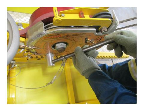
2.1.7. Insert handle into the override-brake hub.
