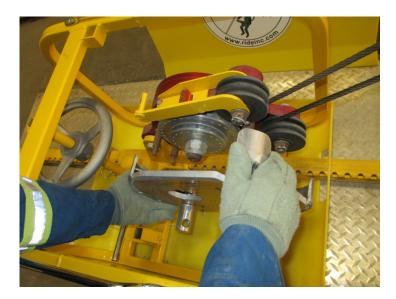
2.1.3. Place the cover onto the Magnegress brake system.
