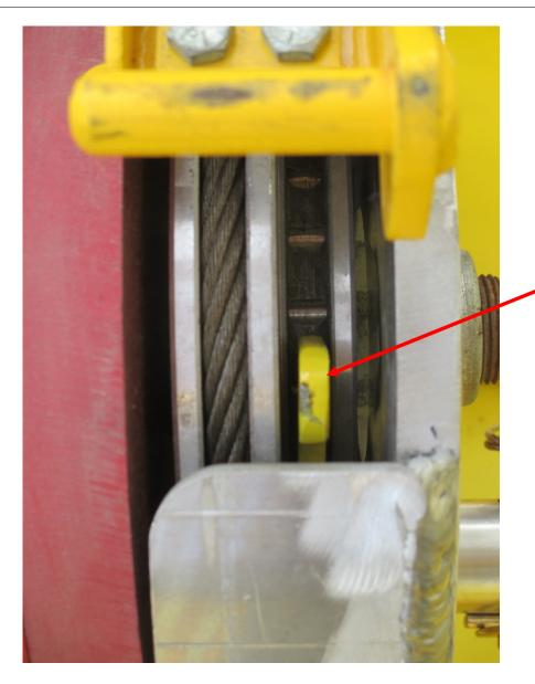
2.1.11. The override brake pad (arrow) should ride the center of the outer sheave.
