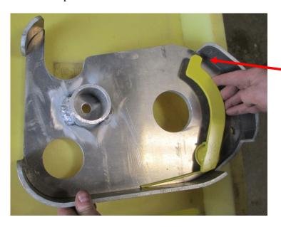
2.1.2. With the cover off check that the brake pad moves freely & that the spring returns the pad to its resting position against the back plate of the cover (arrow).
