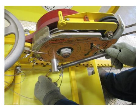
2.1.8. Insert safety pin into the back side of the handle.
