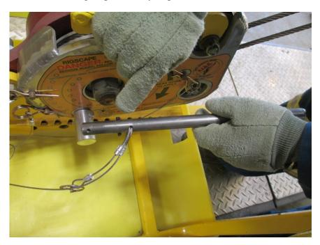
2.1.6. Check to see that the spring pin is properly inserted into the override-brake handle.
