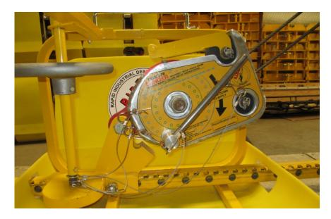
2.1.9. This is a view of the assembled override-brake with handle installed.
